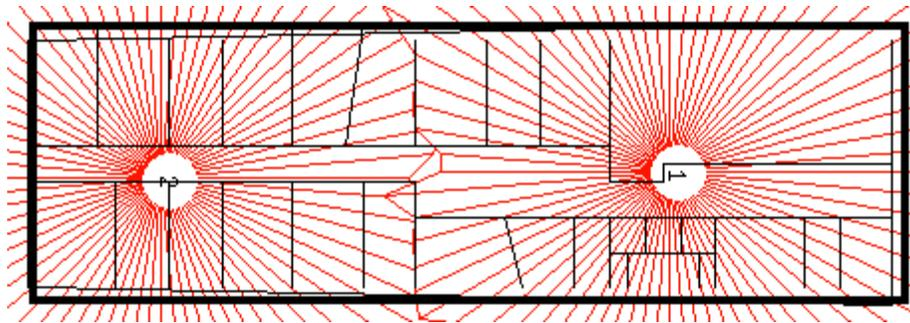
Figure 11: Radio areas of two base station covering the building with stronger walls
