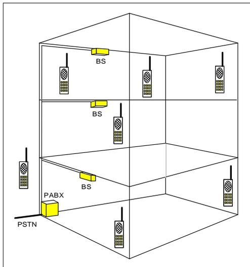
Figure 2: Wireless Private Automatic Branch Exchange (PABX) with Base Stations (BS) and Public Switched Telephone Network (PSTN)
