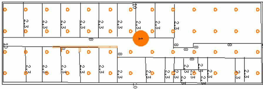
Figure 9: Solution with test point grid size of 4m, possible and chosen positions of base station
