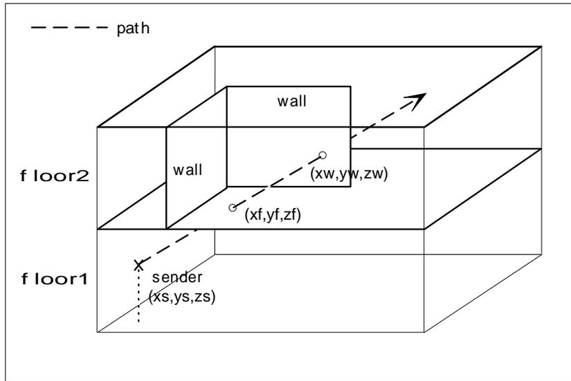
Figure 6: Path from transmitter intersecting a ceiling and a wall
