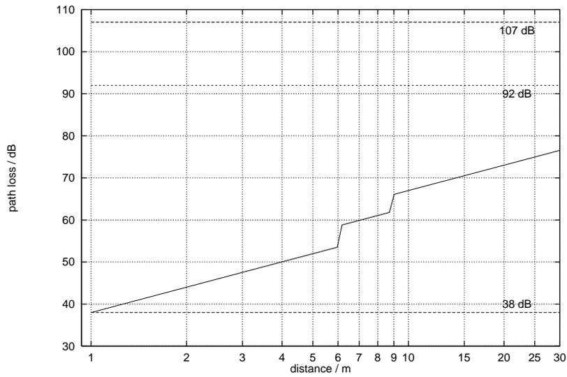
Figure 3: Typical path loss with additional attenuation in 6m and 9m distance due to walls
