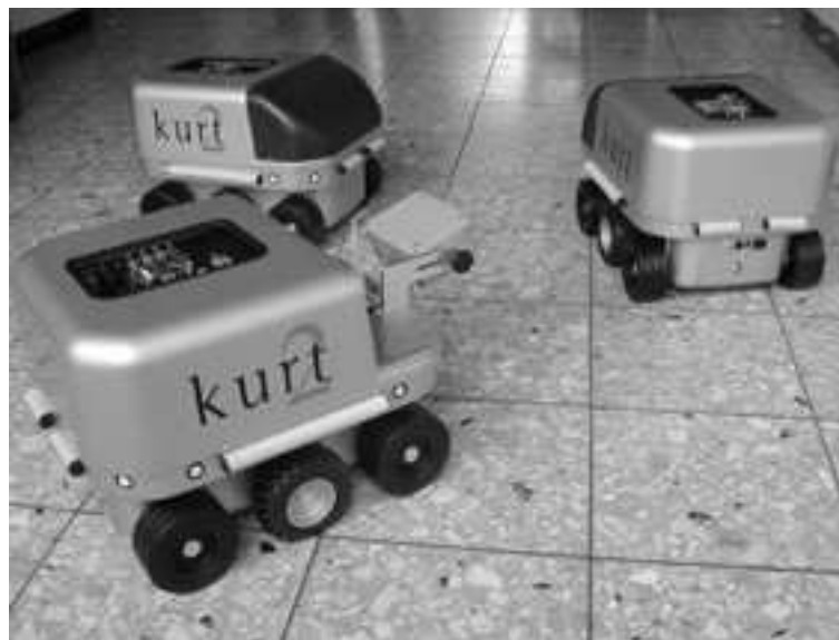
Fig.1 Kurt-2 robots, robot in front carries ICU (courtesy of Michael Mock, Institute of Autonomous intelligent Systems (AiS))
