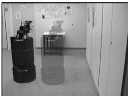
Fig. 7. Experiment showing successful collision avoidance. The obstacle (wall) is detected from the TTC values in the central sector. Left Two superimposed snapshots before the turn. Middle Two
