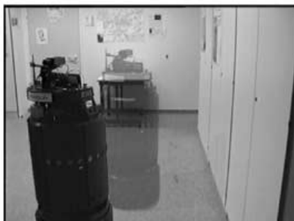
Fig. 7. Experiment showing successful collision avoidance. The obstacle (wall) is detected from the TTC values in the central sector. Left Two superimposed snapshots before the turn. Middle Two
