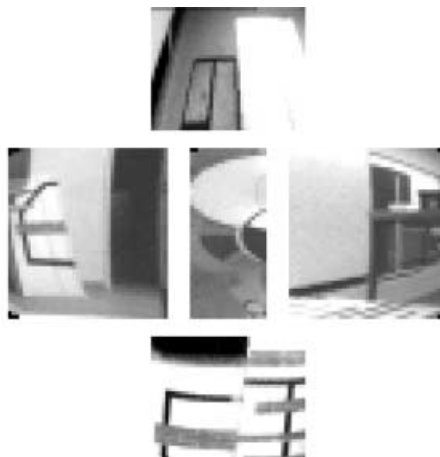
Fig. 4. Image transformation by the PSM. Left Original camera image. Right PSM-transformed image. The data reduction is 10:1 in each of the peripheral sectors and 11:1 in the central complex logarithmic mapping
